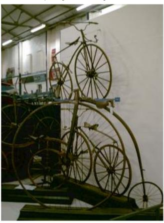
Note how, unusually for an Ordinary, the backbone does not follow the line of the wheel, giving a rather ungainly appearance - almost as if the wheel and backbone were from different machines.
